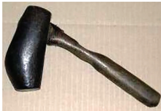
A file cutter's hammer showing wear on the shaft where it was held. To make one file required approximately 2000 strikes
