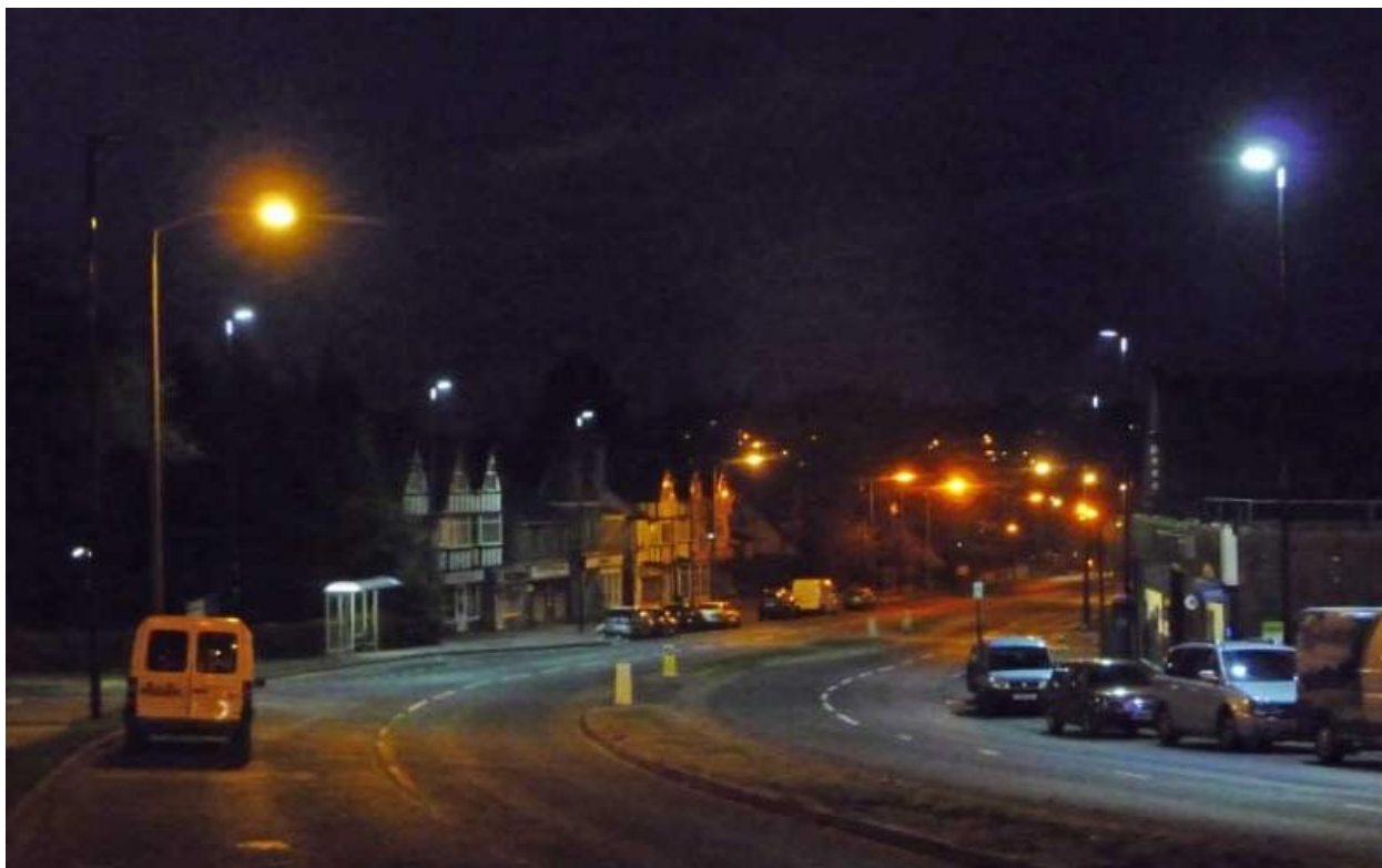
Photograph showing the comparison between the new LED lighting traditional sodium lighting. The lack of glare from the LEDs shows the reduction in light pollution in the sky. Roger Hart
